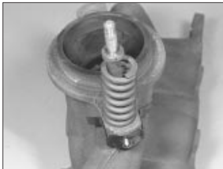
2.2c Showing securing bolts - note coil spring, and shoulder on bolt
