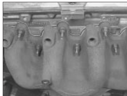
3.13 Exhaust manifold retaining nuts (Zetec engine models)
