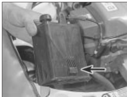
6.13 Undo the retaining screw and withdraw the canister upwards, releasing the tag (arrowed) from its bracket
